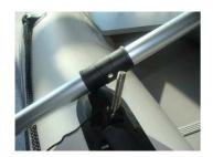
**2.** Insert the screw in the rotating oarlocks in the rudder opening.
