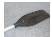
1. Push the safety pushbutton on the rudder tiller down and push the rudder blade up until the safety pushbutton latches the opening provided for this purpose.
