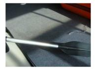
4 .Place both of the oars in the retaining clamps They must latch in under pressure.
